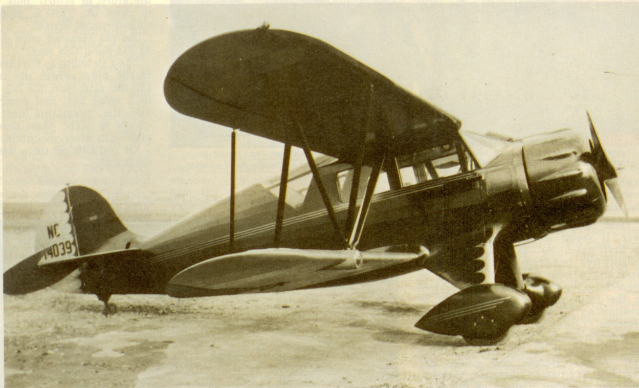
A Waco YKC, representative of most of the Waco cabin models from 1931 through 1936. Smaller lower wings and revised landing gear began to appear on the 1936 models. The triangular windows behind the cabin disappeared by that time. A.U. Schmidt collection
