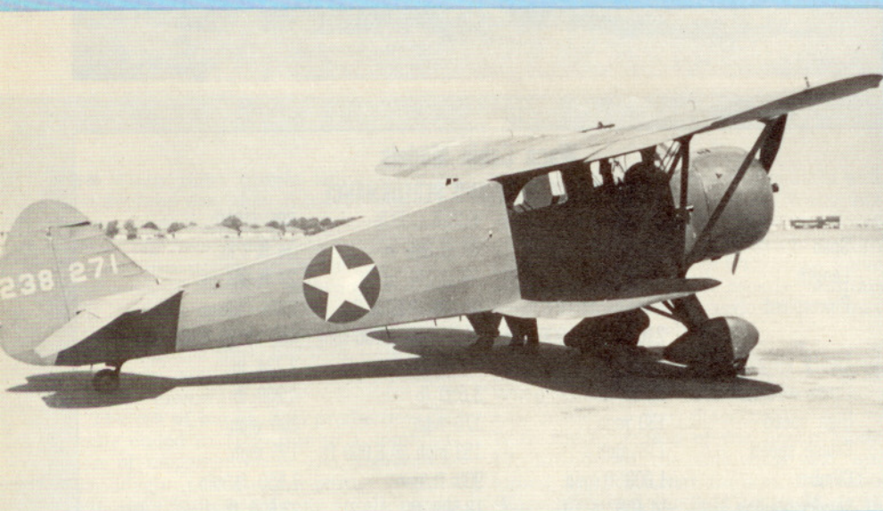
The last and hottest of the cabin Wacos—the 450 hp SRE of the 1940-1941 period. Originally this was NC-31657. It was "drafted" into the Army and became UC-72 42-38271. Note the long, slim fuselage and the use of wires instead of a diagonal strut for wing bracing.
