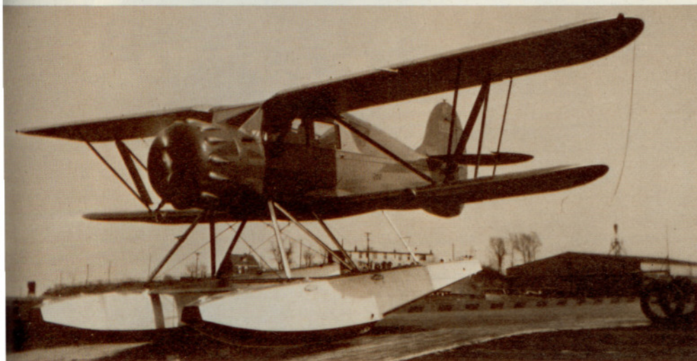
A UKC seaplane of the 1934-1936 era. Note additional fin area added under the fuselage for seaplane operation. On some Wacos, pronounced WAH-cos, a wide fairing on the diagonal of the N-strut could be turned 90 degrees to the airstream to act as a small air brake. Photo by Robert Esposito
